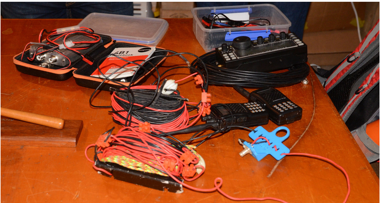
Top: Elecraft KX3 Transceiver. Middle: MX-P50M HF Amplifier. Bottom: Dipole aerials, coax cable and VHF Hand-held radios for local contacts.
