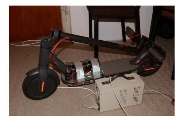
David Probine's test bed for efficiency on the running board. The Supercapacitor Bank and electronics above and battery below.
