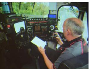
To provide a safe network the communications had to cover the whole network for single manning of a train. The standard adopted requires a signal level of not less than 1 uV for not more
