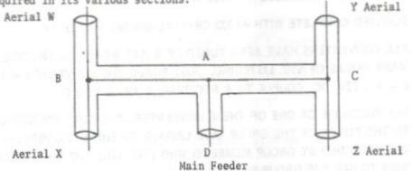
The splitter is usually placed at some central point in the aerial cluster, so that the four aerial feeders connected to B and C are as short as possible, but equal in length.
