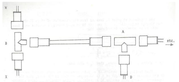
For use with RG - 8A/U and RG - 213/U cable (50-ohms) the tees are UG - 28A/U and the cable connectors are UG - 21B/U not UG - 21D/U which have a poor grip on the cable. AWA and a number of other suppliers have small quantities of these connectors.
