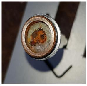
This photo (above) shows the tilt over part of the antenna base where the top of the very rusty spring is a push fit into the hole.
