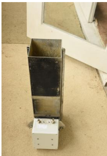
The Septum Feed with LNA mounted on the RX probe
