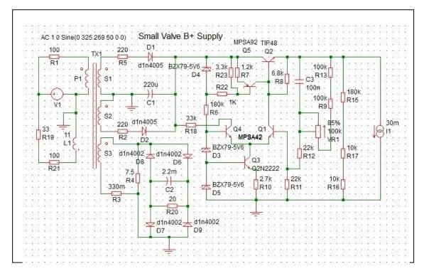
Resistors R9, R13 can be switched in or out to provide 50 V ranges with VR1. C3 helps keep the ripple down. Values were chosen around 5.6 V zeners. R16, R17 represent a 20 V 1 mA meter movement.
