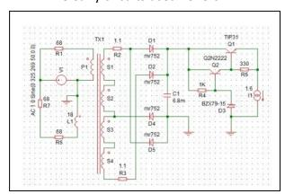
15 V secondaries in parallel have only 2 V headroom at 1.4 A. A 16+ V secondary or a bigger transformer with lower copper loss is required. This transformer has a 2.6 V peak copper loss. The diode loss is 0.8 Vpk x 2.
